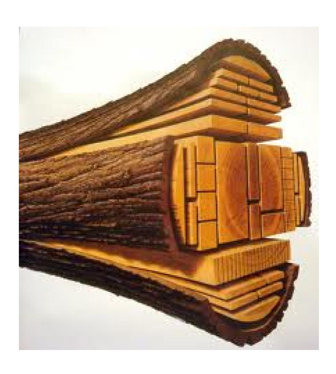
In the process of producing the desired plank of wood, every time the saw kerf (the cut made by a saw in a piece of wood) travels down the rough plank, another centimeter is wasted. To achieve a 1" plank thickness, the mill starts with a bit less than 1.5" to allow for slight warping and some planning, which wastes yet another ½" to 3/8" of wood. In short, the waste is greater than the yield to produce a finished 1" plank and the piece of furniture hasn't even begun.
